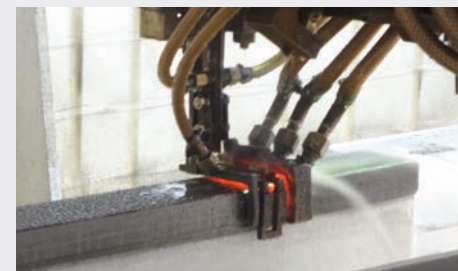
Induction hardened solid box guideways with linear scale feedback on all axes with twin ballscrew design in X & Y axes.
